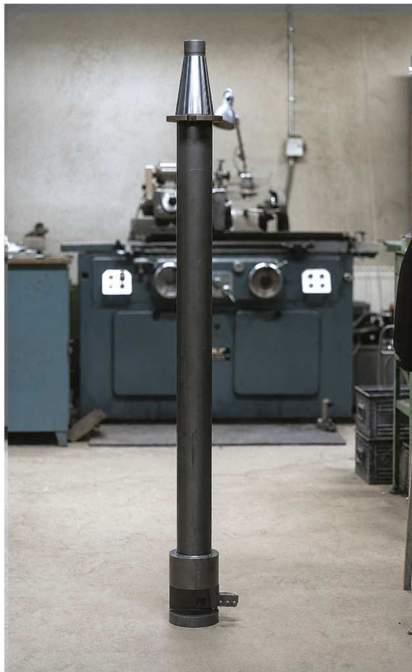
Special tool to operate in a diesel engine block.
